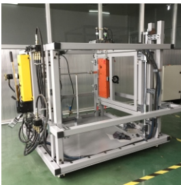
Test devices for ANSI/Euro mortise locks
