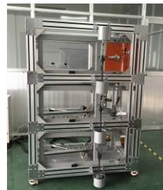
Test devices for ANSI/Euro mortise locks
