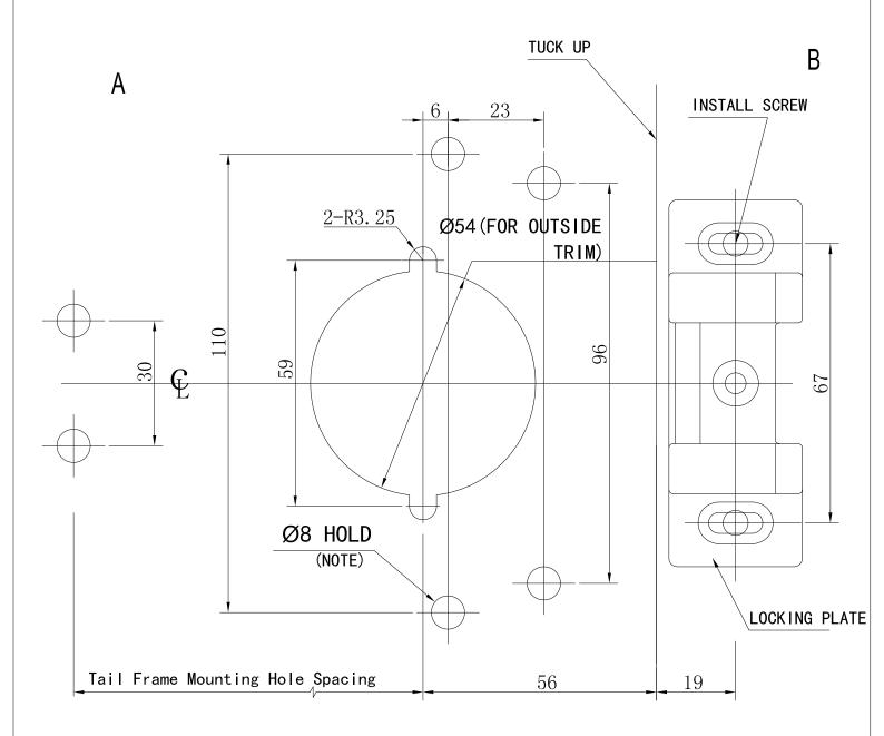
Note:Please confirm whether the door is opened according to the actual products and accessories, When using wooden teeth and tapping screws, it is not necessary to drill  $\phi 8$  holes.
