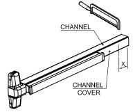
4) CUT THE LENGTH OF THE SCREW ROD AND COVER ACCORDING TO BELLOW LENGTH REQUIREMENT.
