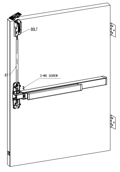
6) INSTALL EACH COVER IN CORRECT SEQUENCE AND TEST THE PRODUCT AT EACH STAGE TO ENSURE CORRECT OPERATION.
